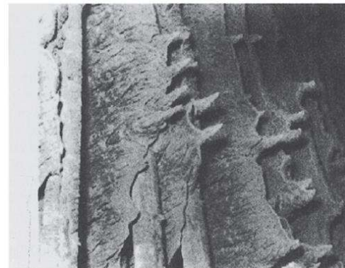
Precipitation fouling of ash particles on superheater tubes.
